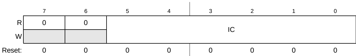
Figure 24-3. I 2 C Frequency Divider Register (I2FDR)
