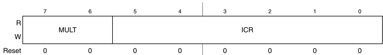
Figure 10-4. IIC Frequency Divider Register (IICF)
