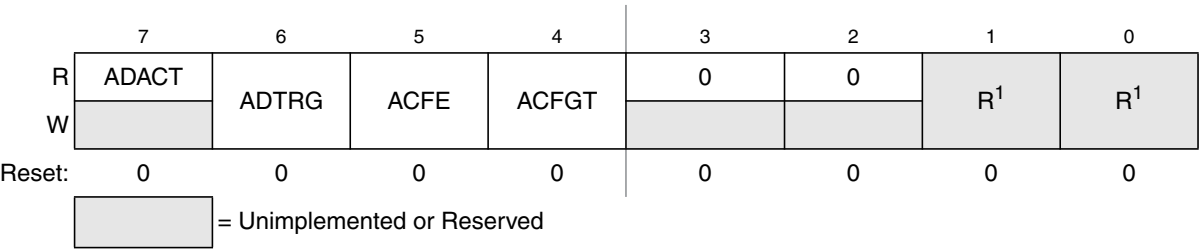
Figure 14-5. Status and Control Register 2 (ADC1SC2)
