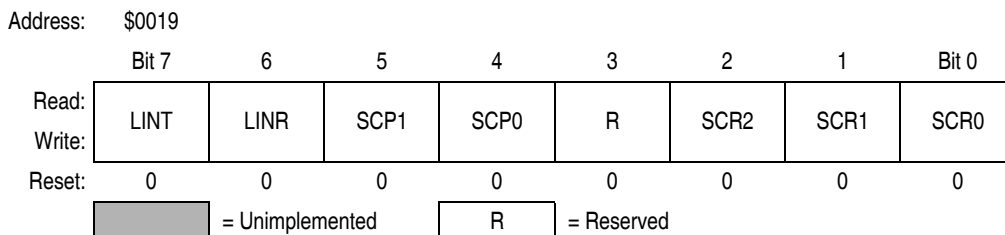
Figure 14-17. ESCI Baud Rate Register (SCBR)
