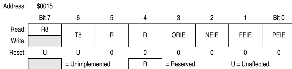
Figure 16-13. SCI Control Register 3 (SCC3)
