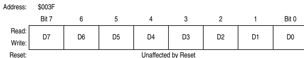
Figure 4-21. BDLC Data Register (BDR)
