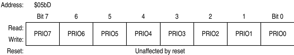
Figure 12-14. Transmit Buffer Priority Register (TBPR)
