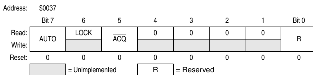
Figure 4-5. PLL Bandwidth Control Register (PBWC)
