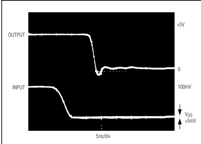
Figure 4. t_{pd-} Response Time to 5mV Overdrive
