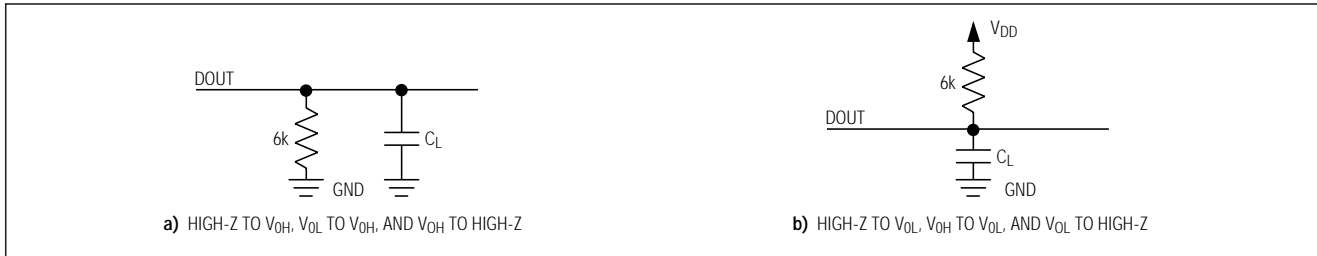
Figure 1. Load Circuits for Enable and Disable Time
