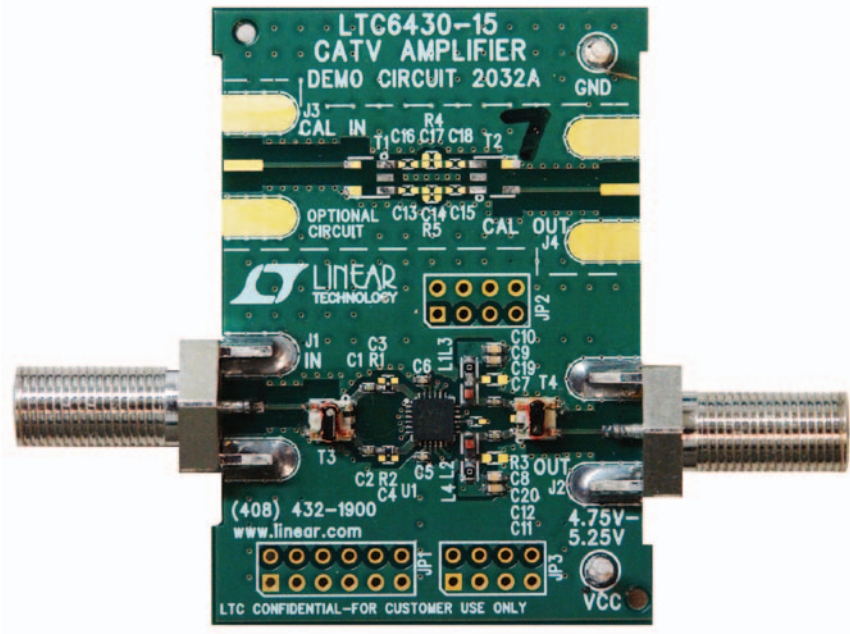
Figure 17. LTC6430-15 CATV Evaluation Board
