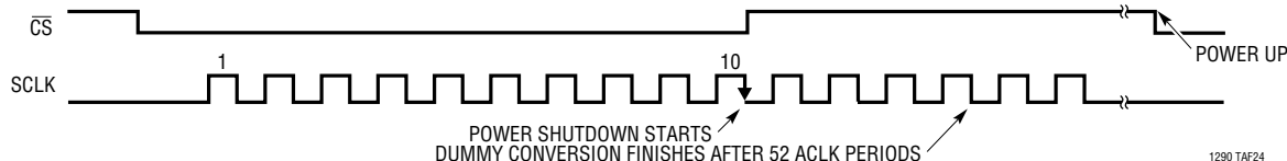
Figure 24. Power Shutdown Timing
