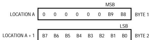
D_{OUT} from LTC1091 Stored in MC68HC05C4 RAM
