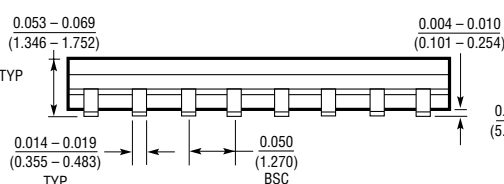
S Package 16-Lead Plastic Small Outline (Narrow 0.150) (LTC DWG # 05-08-1610)
