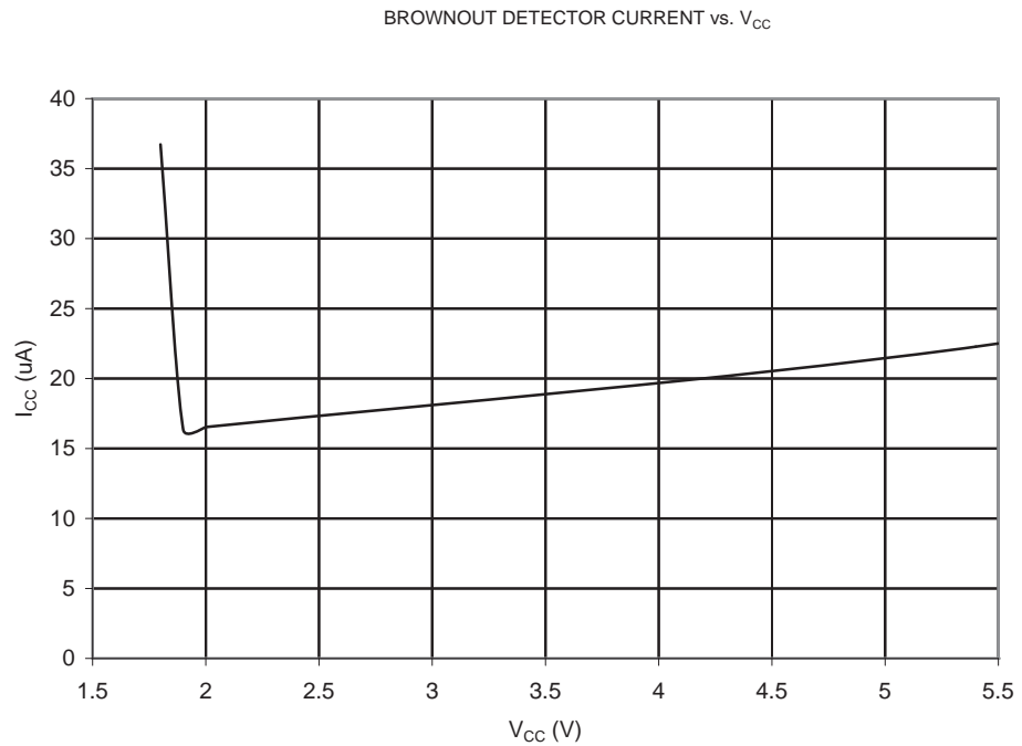
Figure 20-69. Brownout Detector Current vs. V_{CC}
