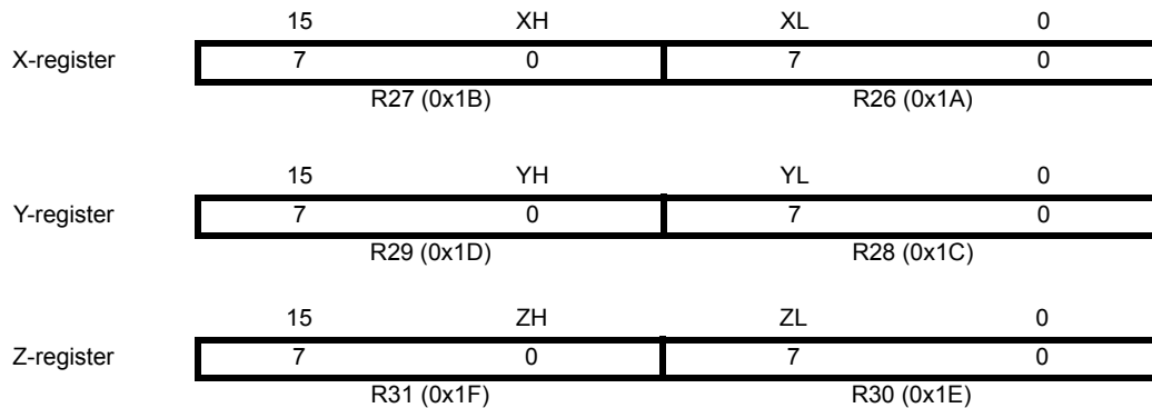
Figure 5-3. The X-, Y-, and Z-registers
