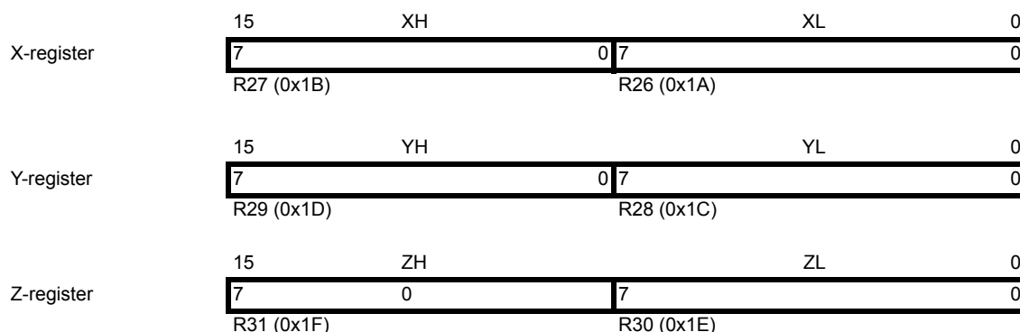
Figure 2-3. The X-, Y-, and Z-registers
