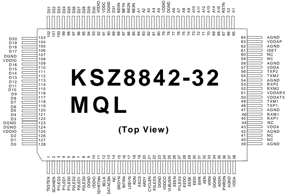
Figure 5. Standard – KSZ8842-32 MQL 128-Pin PQFP (Top View)
