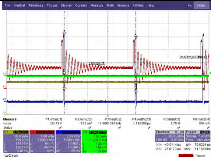
Fig. 6G - 90Vac in, 16Vout / no load (recaptured – closer view)
