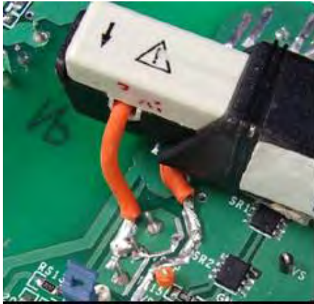
Fig. 4B Recommended probing of secondary current waveform.
