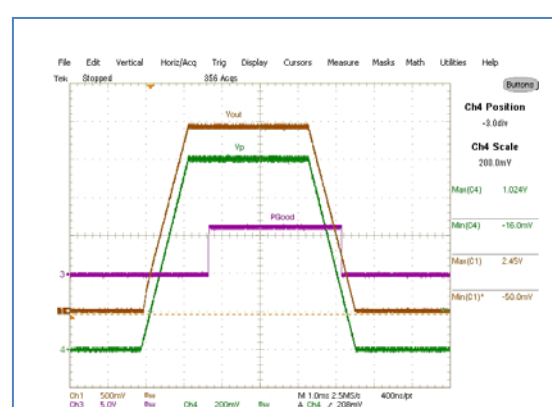
Figure 44: Voltage tracking using Vp pin Ch1:V out , Ch3:P Good , Ch4:V p
