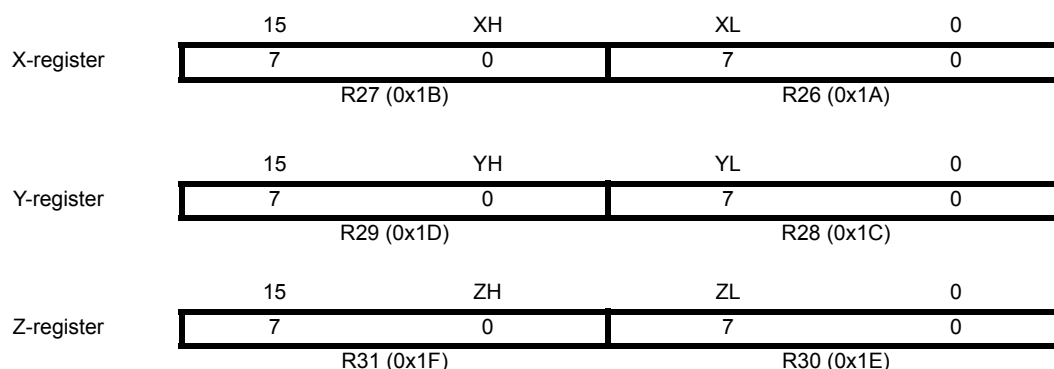
Figure 4-3. The X-, Y-, and Z-registers
