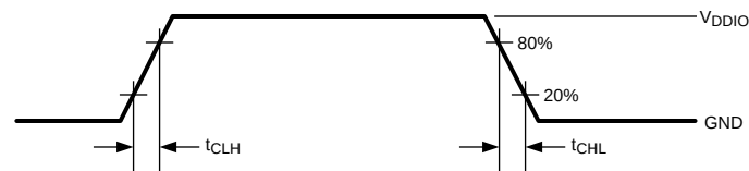
Figure 1. LVCMOS Transition Times
