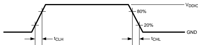
Figure 4. LVCMOS Transition Times
