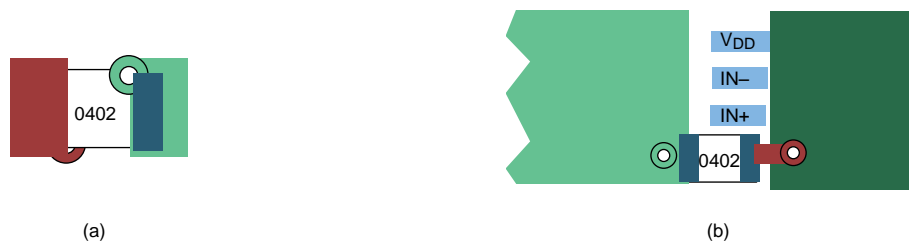
Figure 21. Typical Decoupling Capacitor Layouts
