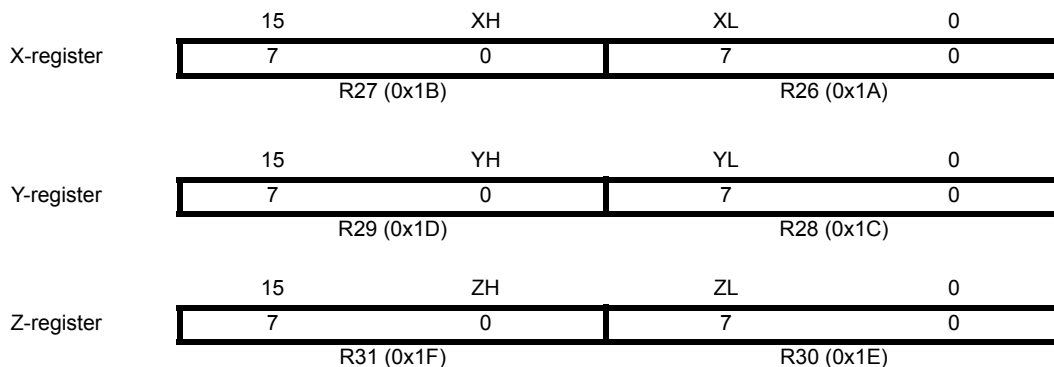
Figure 4-3. The X-, Y-, and Z-registers
