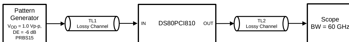
Figure 10. Test Setup Connections Diagram
