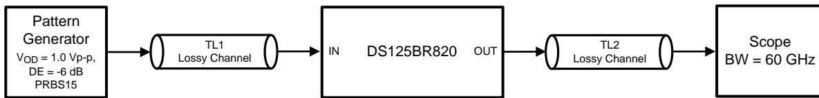
Figure 10. Test Setup Connections Diagram
