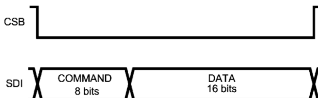
Figure 9. SPI Command and Data Words
