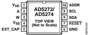
Figure 4. MSOP Pin Configuration
