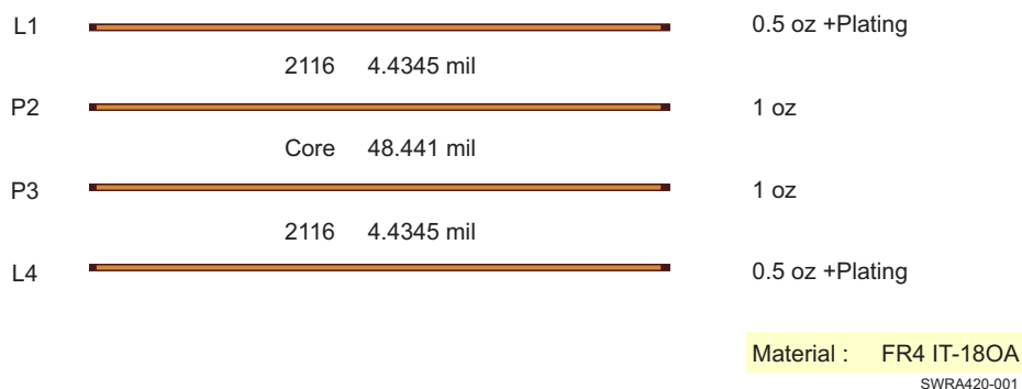
Figure 1. PCB Stack-Up
