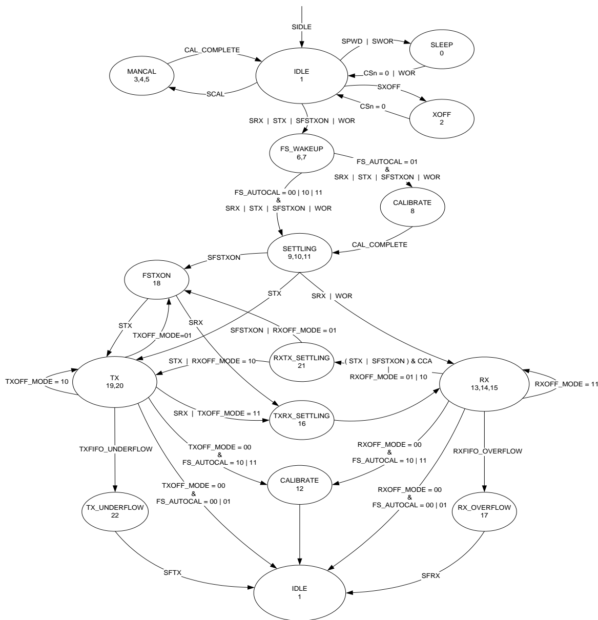
Figure 25: Complete Radio Control State Diagram
