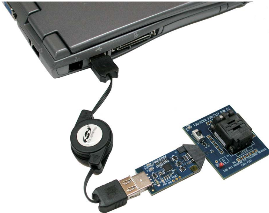
Figure 5. ToolStick Socket Platform Connected to PC
