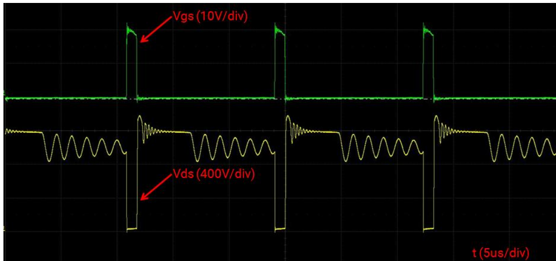
Figure 5 Switching waveforms V_{gs} and V_{ds} of the SiC MOSFET.
