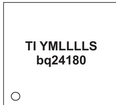
CHIP SCALE PACKAGE (Top Side Symbol For bq24180)
