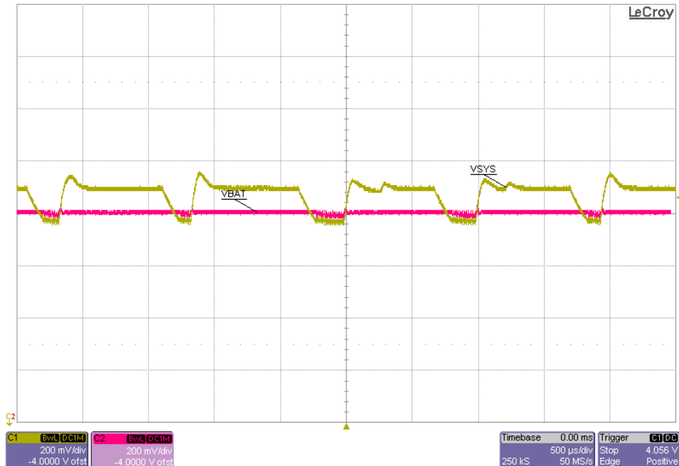
Figure 16. V(SYS) when Reverse Boost Prevention Circuit is Active
