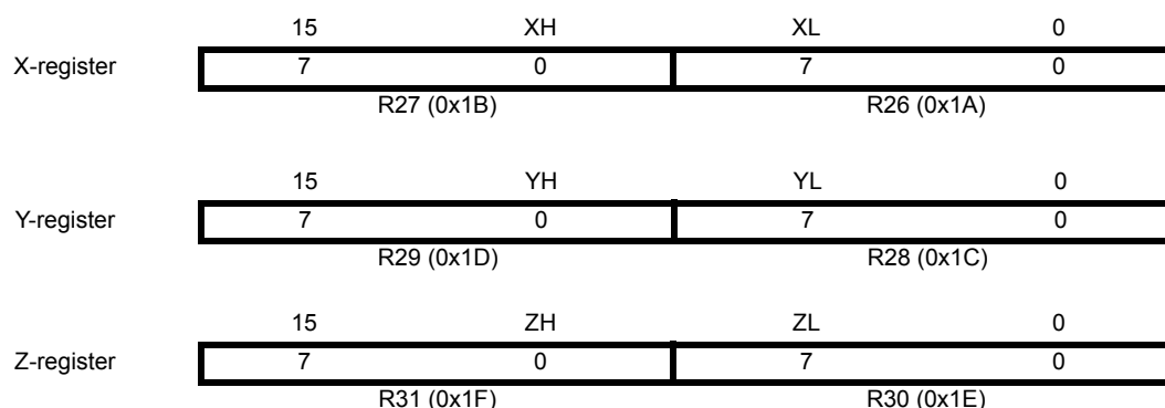
Figure 4-3. The X-, Y-, and Z-Registers
