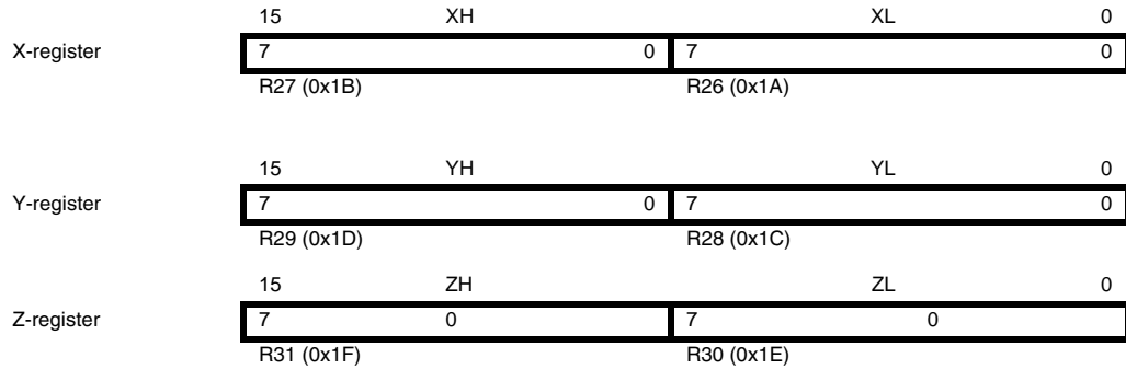
Figure 4-3. The X-, Y-, and Z-registers
