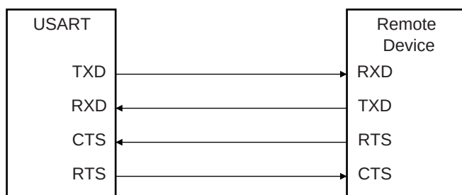
Figure 25-26. Connection with a Remote Device for Hardware Handshaking
