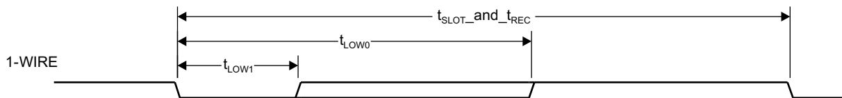
Figure 5-118. 1-Wire Write Bit Timing (Command/Address or Data)
