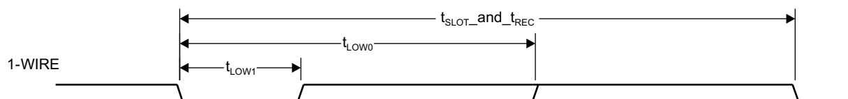
Figure 5-118. 1-Wire Write Bit Timing (Command/Address or Data)
