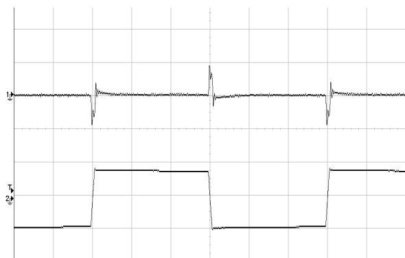
Figure 5 Dynamic response for 25% load step (25% ~ 50% ~ 25%) and 0.1A/ \mu s slew rate, (1ms/div), see Figure 11 for test configuration; CH1-output voltage (50mV/div); CH2-output current (10A/div)
