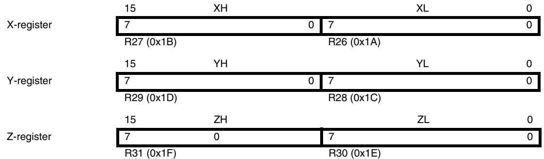
Figure 4-4. The X-, Y-, and Z-registers
