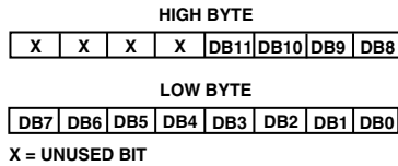
Figure 30. Data Format for AD5343
