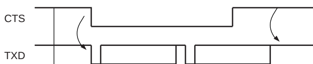
Figure 38-28. Transmitter Behavior when Operating with Hardware Handshaking
