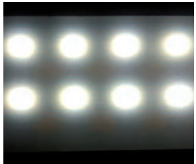
Infineon solution with XMC1000. Flickering (40–50 kHz) is neither visible nor detectable by HD cameras.
