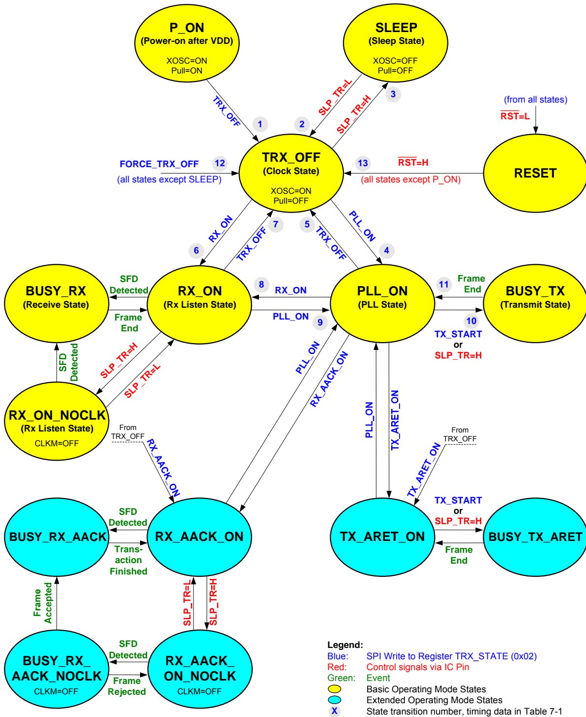
Figure 7-5. Extended Operating Mode State Diagram
