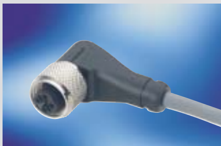
Female cable connector, right angled, unshielded with anti-vibration coupling nut and overmolded cable A-coded
