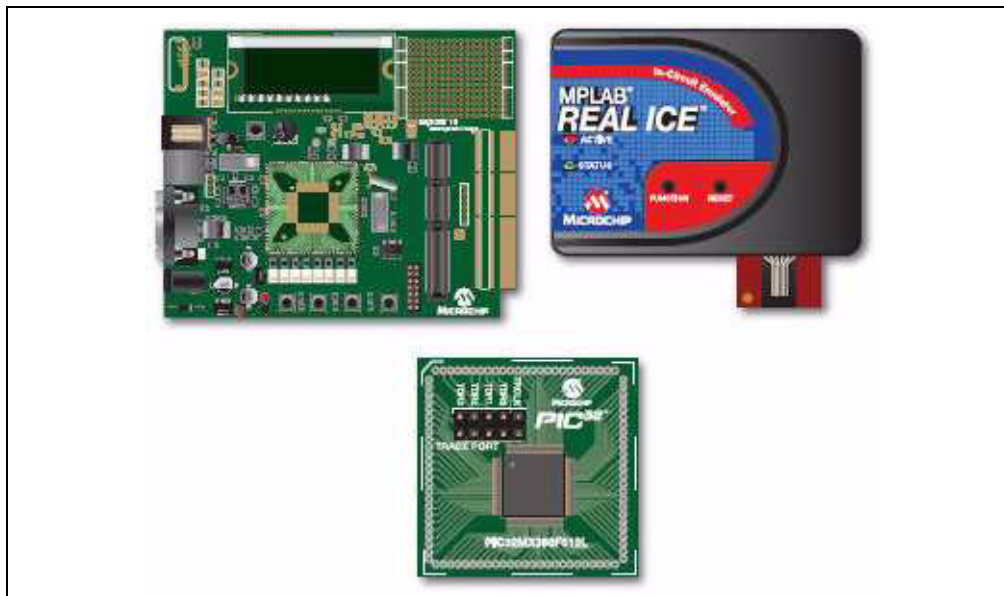
FIGURE 5-11: EXPLORER 16, MPLAB ® REAL ICE ™ AND PIC32MX360F512L PIM
