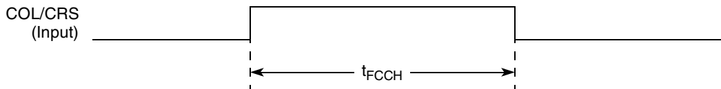
Figure 26. Ethernet Collision AC Timing Diagram (FCC)
