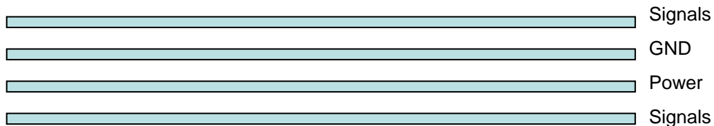
Figure 21: Typical 4-layer PCB construction
